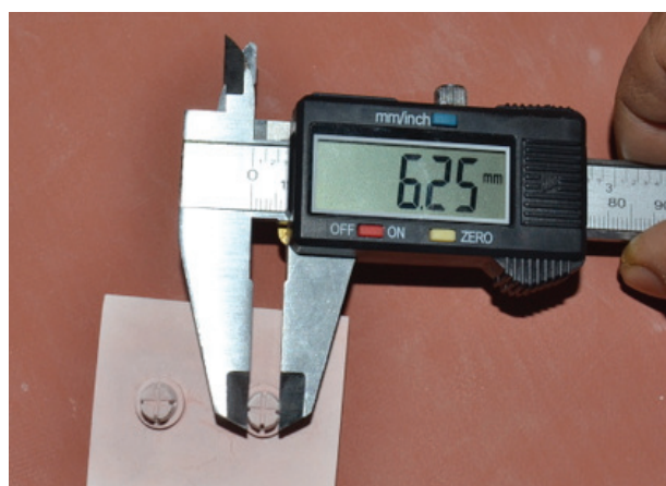
Figure 8: Measurement of mesio distal (MD) dimension with digital Vernier caliper
