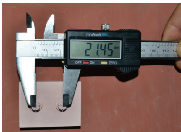
Figure 7: Measurement of interpretation dimension (IP) with digital Vernier caliper
